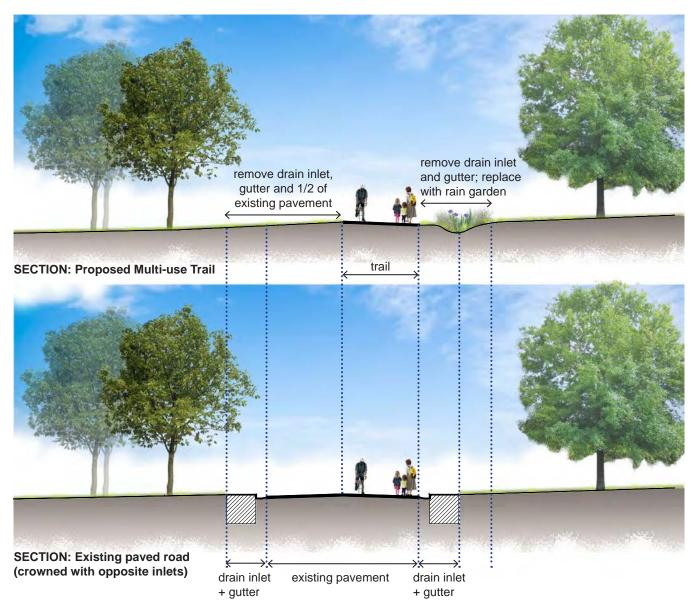
Figure 33. Section drawings showing the reduction in width of existing streets to support multi-use paths
